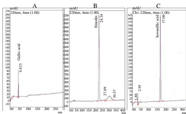
Figure 1. Chromatograms of HPLC analyses of standards of compounds.
